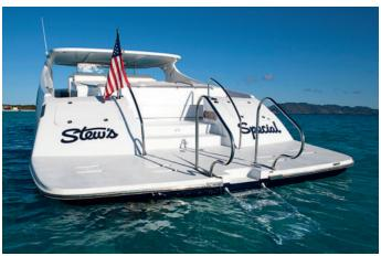
Custom-built stairs deploy from the swim platform to help passengers ease their way in and out of the yacht
