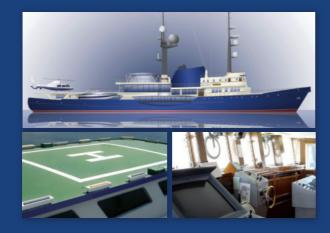
Length Overall: 77.4 m Beam: 13.2 m Draught: 5.78 m Cruising Speed: 15 kn Main Engines: 2 x 4400 bhp
